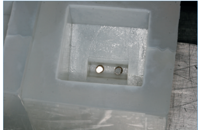
Figure 9. Different steps on the model materialization: The assembly showed on Figure 4 placed into the silicon mould.
