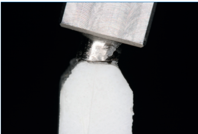
Figure 17. Damage found on the completed static test. Compared with figure 16 it is possible to observe the same tendency.
