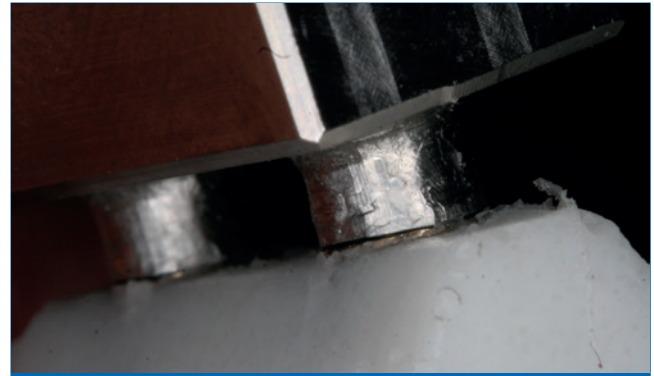
Figure 25. Correspondence between the damage sequences on both studies: 4000 N on interrupted static test (prosthetic framework).
